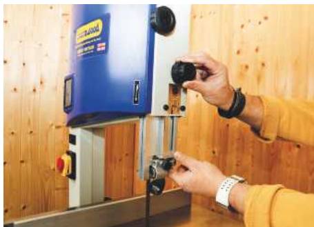
▲ The height post is set with the double-function knob
